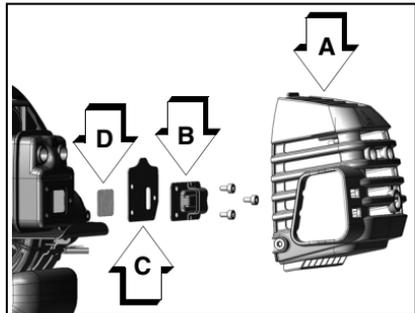
**Note:** When cleaning carbon deposit, be careful not to damage the catalytic element inside muffler.
