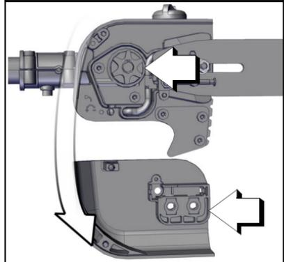
4. Hold the bar nose up. Install guide bar cover (D). Install the guide bar nuts (A). Tighten the rear nut first, then tighten the front nut. Install and tighten the guide bar cover screw (B)
