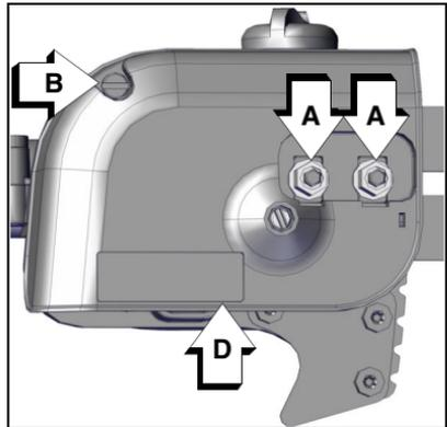
3. Gently brush debris from inside guide bar cover and from around sprocket.
