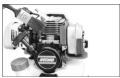
6. Remove grass and leaves from the grid between the recoil starter and fuel tank.
