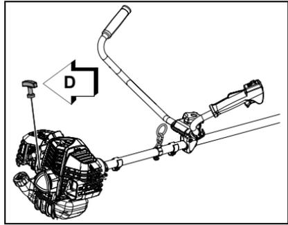
Note: If engine does not start after five pulls, use Cold Start Procedure.
