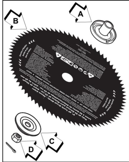
3. Align hole in upper plate with notch in gear housing, and insert locking tool (E) to prevent splined shaft from turning. Tighten the 10 mm nut securely.
