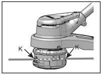
Hold trimmer head while turning knob clockwise to wind line onto spool until about 13 cm (5 in.) of each line remains exposed.
