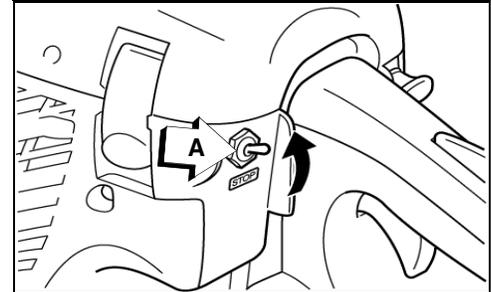
4. Securely hold the chain saw as shown and pull starter handle.
