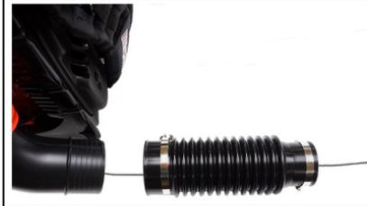
4. Assemble flexible pipe to elbow (D) on blower. Position clamp with cable guide loop (G) on outside of flexible pipe and tighten clamp.
