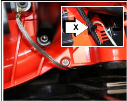
3. Insert anti-static wire through flex tube. Leave enough slack in anti-static wire to allow for full rotation of elbow.
