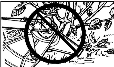
**8 Tooth Weed/Grass Blade** is designed for grass, garden debris and thick weeds up to 19 mm (3/4 in.) diameter. DO NOT use this blade for brush or heavy woody growth.
