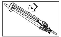
Hold blade adjustment handle (B) and compress blade lock levers (C) and (D) together. Rotate blade to desired position. Release levers to lock blade.
