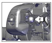
spin the engine. Do not pull the rope out to end stop.
