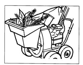
5. Material consisting mostly of leaves can be raked next to the hopper with the hopper turned to the side (perpendicular) and the leaves will be drawn into the machine and shredded.
