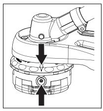
3. Insert one end of trimmer line into an eyelet, and push line equal distance through trimmer head.
