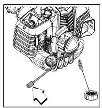
When the inside of the fuel tank is dirty, rinse the tank out with gasoline to clean it.
