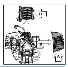
DO NOT use a metal scraper to remove dirt from the cylinder fins.
