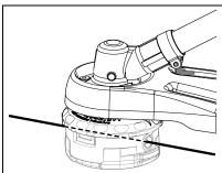
4. Hold trimmer head while turning knob clockwise to wind line onto spool until about 13 cm (5 in.) of each line remains exposed.
