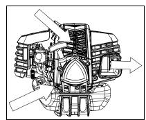
· Dust and grass build up on the outside of the cylinder. This build up insulates the engine and prevents the heat from leaving.
