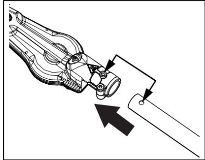
5. Install locating bolt (A). Tighten clamping bolt (B).
