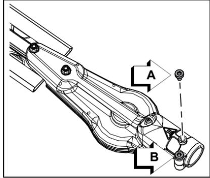
3. Align locating hole in gear housing with locating hole in drive shaft.
