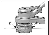
Hold trimmer head while turning knob clockwise to wind line onto spool until about 13 cm (5 in.) of each line remains exposed.
