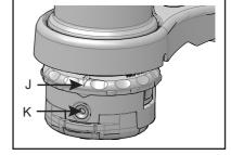
Insert one end of trimmer line into an eyelet (K), and push line equal distance through trimmer head.
