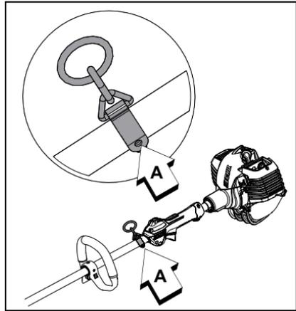
3. Slide harness clamp up or down until unit balances with head or blade  $200\text{ mm} \pm 100\text{ mm}$  (8 in.  $\pm$  4 in.) from the ground.
