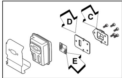
5. Replace screen if it is cracked, plugged, or has holes burned through.
