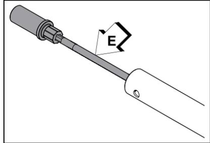
8. Install and tighten set screw (D), and tighten clamping screw (C).
