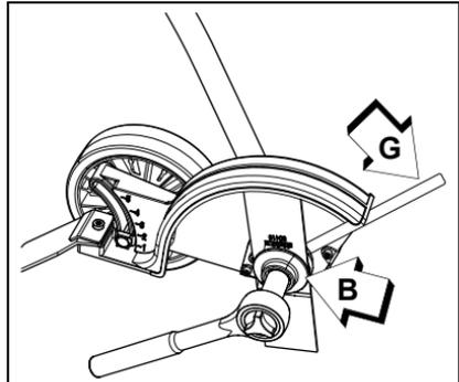
2. Align hole in inner blade adapter (B) with notch in gear housing, and insert locking tool (G) to prevent PTO shaft (C) from rotating.
