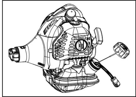
Note: Federal EPA regulations require all model year 2012 and later gasoline powered engines produced for sale in the United States to be equipped with a special low permeation fuel supply hose between the carburetor and fuel tank. When servicing model year 2012 and later equipment, only fuel supply hoses certified by EPA can be used to replace the original equipment supply hose. Fines up to \$37,500 may be enforced for using a non-certified replacement part.
