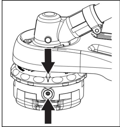
3. Insert one end of trimmer line into an eyelet, and push line equal distance through trimmer head.
