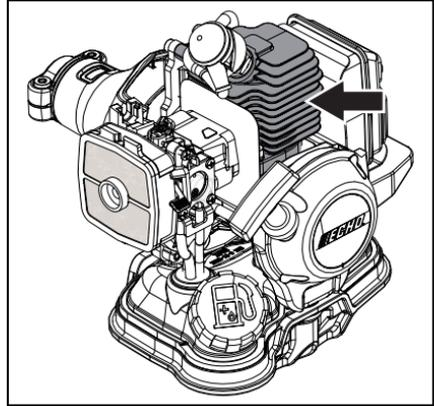
6. Remove grass and leaves from the grid between the recoil starter and fuel tank.
