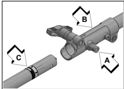
5. Rotate locator pin (A) one-quarter turn clockwise to engage lower shaft hole. Make sure locator pin is fully engaged by rotating the lower drive shaft. Locator pin should snap flush in coupler. Full engagement will prevent further shaft rotation.
