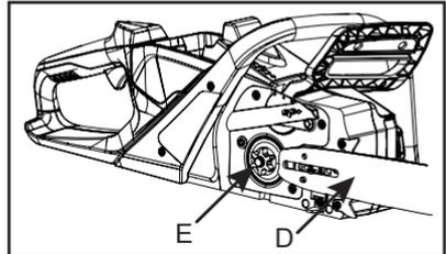
4. Install saw chain as shown (ensure cutters are pointing in the right direction).
