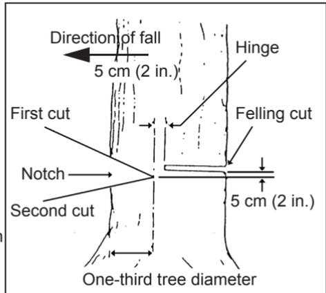
The remaining wood between the notch cut and felling cut about 5 cm (2 in.) will act as a hinge when the tree falls, guiding it in the desired direction. When the tree starts to fall, kill the motor, place the saw on the ground and make your retreat quickly.
