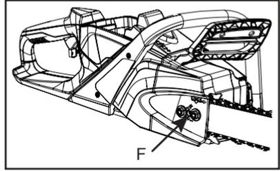
9. Tighten nuts with the guide bar nose held up.
