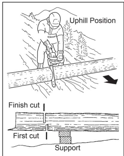
Keep in mind that the wood is heavy and that it will bend and pinch the saw if improperly supported. The trunk will weaken at the point where you make the cut unless the tree is lying on perfectly flat ground or supported as shown. If you make the cut with the tree on the ground, don't let the saw's chain dig into the earth; it is harmful for the saw, and you stand a good chance of being struck by flying debris.
