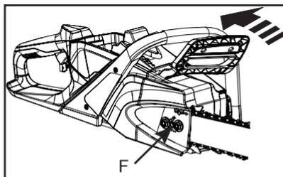
3. Tighten sprocket cover nuts with the bar nose held up and under tension.
