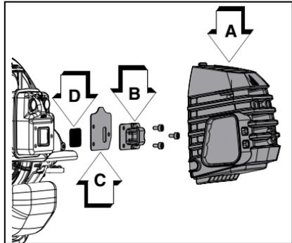
6. Replace screen if it is cracked, plugged, or has holes burned through.
