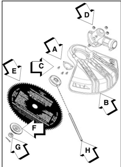
4. Install blade (E) on upper plate pilot. The rotation arrows on the blade must match the rotation arrow shown on the debris shield. Secure blade with lower plate (F), and 10 mm left-hand threaded nut (G). Turn nut counterclockwise on power take off shaft to tighten.
