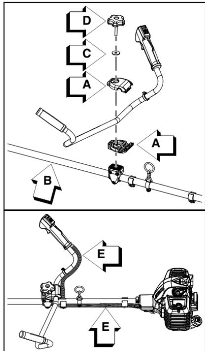
2. Route throttle linkage and ignition lead assembly (E) along shaft and clip as shown.
