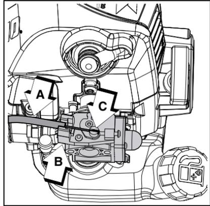
Note: The throttle linkage must be adjusted by moving the adjustment nut. Consult with your dealer for correct adjustment procedure.
