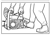
8. Push choke control knob all the way IN (OPEN [] ∤ ]]choke position).
