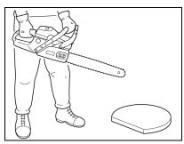
2. Move chain brake lever fully REARWARD to UNI OCK chain. brake.
