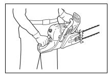
Start the engine, see that it is running properly. Squeeze the trigger to open the throttle wide open and start the cut. If the chain is properly sharpened, the cutting should be relatively effortless. It is not necessary to press down hard to make the saw cut. Pushing the saw too hard will slow the engine and cutting will actually be more difficult.
