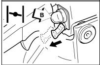
7. Securely hold the chain saw and pull starter handle several times until first starting sound.
