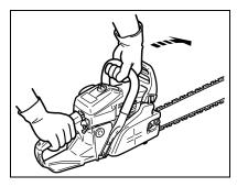
3. Move stop switch (A) to "RUN" position.
