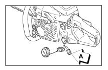
Pull filter out through gas port, and inspect filter.
