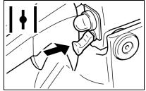
Do not allow recoil handle to snap back against the case.
