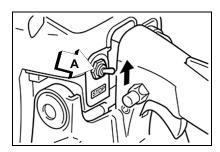
Securely hold the chain saw as 4. shown and pull starter handle.
