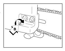
Tighten nuts with the bar nose held up.
