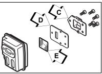
3. Use a wood or plastic scraping tool to clean deposits from cylinder exhaust port (C).
