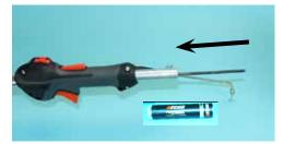
28. Connect the two (2) Ignition Leads between the Control Handle and engine then slide engine onto Main Pipe assembly.
