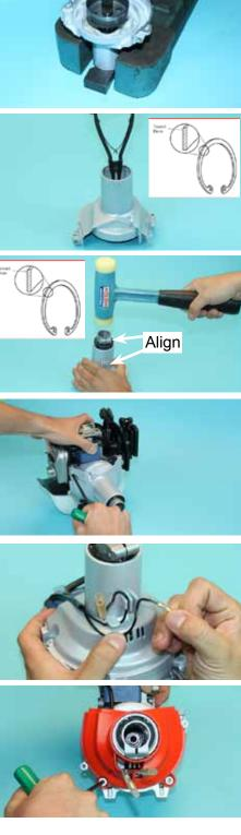
20. Install Engine Cover with two (2) T27 screws using torx driver: rear center, and top left.
