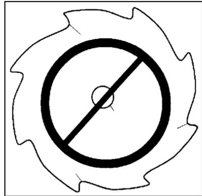
1. File each tooth at a 30 degree angle a specific number of times, e.g., 4 strokes per tooth. Work your way around the blade until all teeth are sharp.
