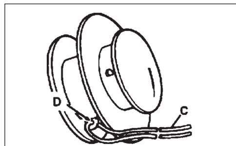
3. Hold the spool, opening toward you. Place index finger between the two strands and wind line, tightly and evenly, in direction of arrow marked "CC".
