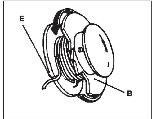
5. Feed ends of line through housing eyelets (F) and place spool (B) over drive (G). Align pegs (H) on drive with notches in spool and push spool into drum.
