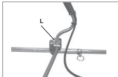
12. Route throttle linkage and ignition lead assembly around front of U-Handle bracket and clip to drive shaft as shown.
