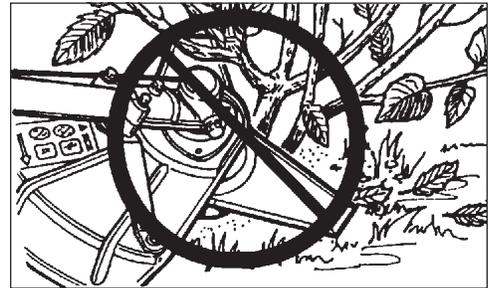
**ss8 Tooth Weed/Grass Blade** (P/N 69600120331) is designed for grass, garden debris and thick weeds. **DO NOT** use this blade for brush or heavy woody growth, 3/4" in. (19 mm) diameter or larger. U-Handle / Blade Conversion Kit P/N 99944200521 is required for use with this blade.
