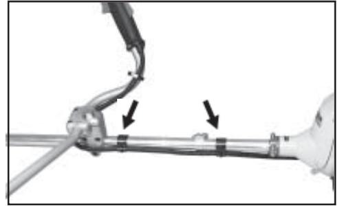
13. Place throttle linkage (E) through adjustment fixture (F) and install wire end into large carburetor throttle swivel hole (D). Check throttle for freedom of movement and that wide open throttle / low idle extremes are adjusted properly. The throttle linkage must be adjusted by moving the adjustment fixture (F). Consult with your Echo Dealer for correct adjustment procedure.
