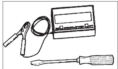
1. Check idle speed and reset if necessary. If a tachometer is available, idle speed screw (A) should be set to the specifications found on page 13 "Specifications" of this manual. Turn idle screw (A) clockwise to increase idle speed; counter clockwise to decrease idle speed.
