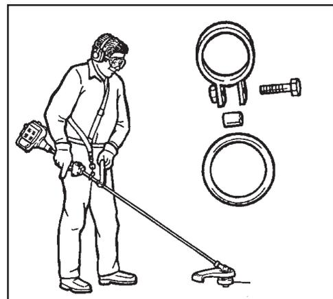
4. Install front handle, gear housing and shield.
