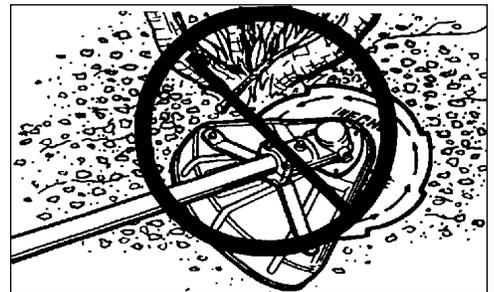
**80 Tooth Brush Blade** is designed for cutting brush and woody growth up to 64 mm (1/2 in.) diameter.
