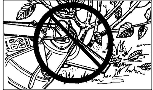
**8 Tooth Grass and Weed Blade** is designed for grass, garden debris and thick weeds up to 19 mm (3/4") diameter. **DO NOT** use this blade for brush or heavy woody growth.
