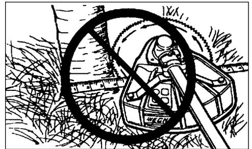
**22 Tooth Clearing Blade** is designed for dense thickets and saplings up to 64 mm (2-1/2 in.) diameter.
