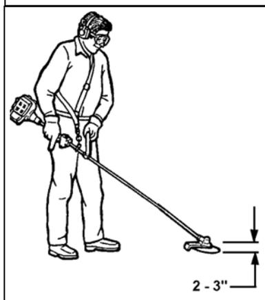
Note: In case of Emergency, the trimmer/brushcutter can be released from the harness by pulling up on the quick-release collar.
