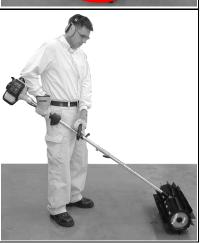
5. Debris may be swept out and away from corners by turning unit over to reverse paddle direction. Grip unit securely using both hands. Operate throttle trigger with thumb of right hand. For extended use, reposition front handle to allow comfortable grip. Return handle to normal position for regular operation.
