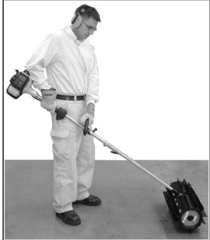
5. Debris may be swept out and away from corners by turning unit over to reverse paddle direction. Grip unit securely using both hands. Operate throttle trigger with thumb of right hand. For extended use, reposition front handle to allow comfortable grip. Return handle to normal position for regular operation.
