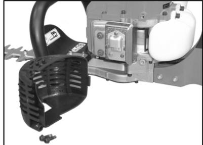
4. Remove exhaust guide (A), gasket (B), and screen (C) from muffler body.
