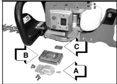
Note: When cleaning carbon deposits, be careful not to damage the catalytic element inside muffler.
