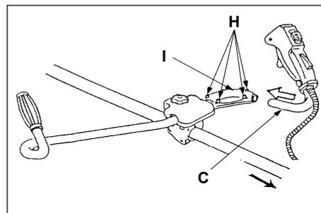
6. Secure the right hand U-handle by tightening 4 right handle assembling bolts (H) loosely.
