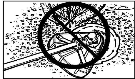
**80 Tooth Brush Blade** is designed for cutting brush and woody growth up to 13 mm (1/2 in.) diameter.
