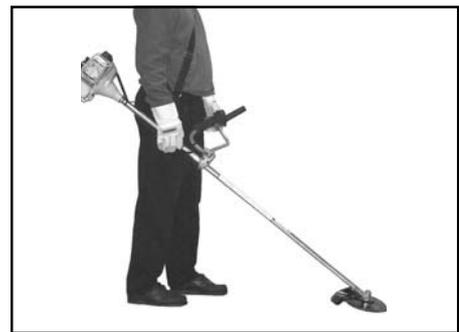
During blade operation, the same fatigue reduction is achieved. Safety to the operator is also enhanced by reducing the possibility of blade contact with the operator's hands and feet by restricting trimmer movement
