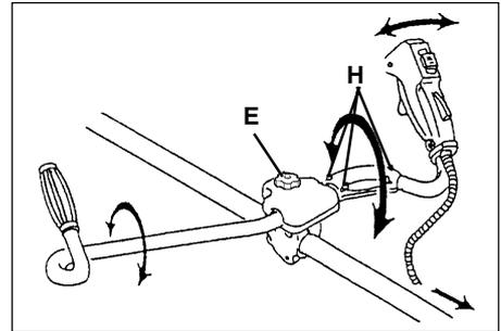
8. Route throttle linkage and ignition lead assembly along shaft and clip as shown.
