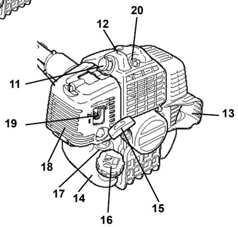
1. **POWER HEAD** - Includes the Engine, Clutch, Fuel System, Ignition System and Recoil Starter.
