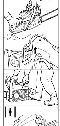
4. Securely hold the chain saw as shown and pull starter handle.
