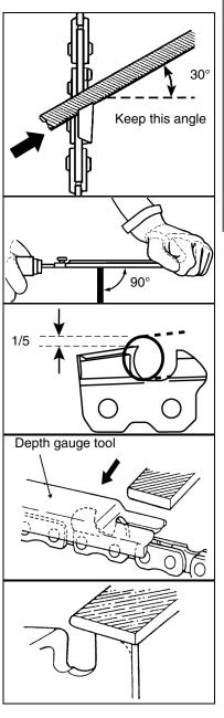
When setting of the chain is finished, soak it in oil and wash away filings completely before using.
