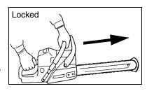
Do not attempt to operate the engine with the brake locked.
