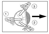
by drawing the saw forward in the cut to reach the hinge.
