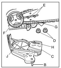
Install sprocket guard (C) over guide bar studs. Ensure chain tension adjuster pin (H) fits into the guide bar adjuster hole (G), brake band (J) is positioned around clutch drum. Install knob (D) and tighten securely with bar nose held up.
