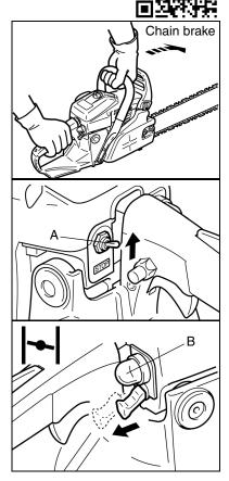
7. Securely hold the chain saw and pull starter handle several times until first starting sound.
