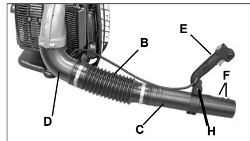
5. Assemble flexible pipe (B) to elbow (D) on blower and tighten clamps (A). Position guide loop (G) on inside (blower side) of flexible tube.
