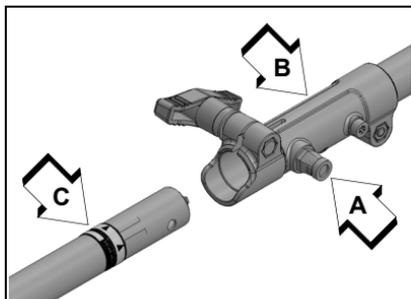
5. Rotate locator pin (A) one-quarter turn clockwise to engage lower shaft hole. Make sure locator pin is fully engaged by rotating the lower drive shaft. Locator pin should snap flush in coupler. Full engagement will prevent further shaft rotation.
