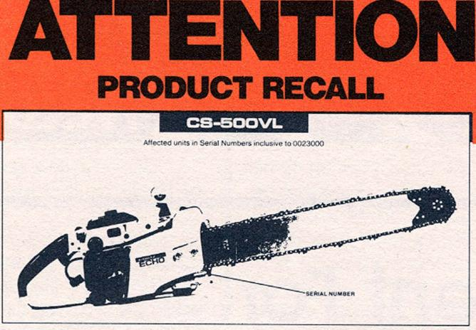
Echo has been advised of injuries sustained by the operators of the model CS-500VL due to fracture of the flywheel at high speed. Laboratory analysis and investigation of units in field service have indicated that the failures have been caused by the use of the wrong tools and techniques in removing the flywheels (see fig. A-B).
