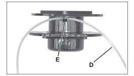
Hold spool with the tap knob in your hand and opening toward you. Place index finger between the two lines, and wind line clockwise tightly and evenly.
