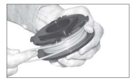
When approximately 15-20 cm (6-8 in.) of line remains, place lines in spool notches (F).
