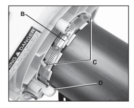
4. Align grooves in discharge elbow with pegs on blower, and slide elbow (D) on to blower. Turn elbow counterclockwise to lock in place. Elbow must angle back toward operator position as shown.
