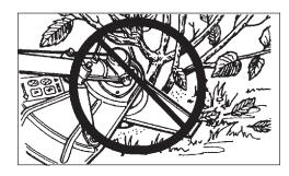
8 Tooth Weed/Grass Blade (P/N 69600120331) is designed for grass, garden debris and thick weeds. DO NOT use this blade for brush or heavy woody growth, 19 mm (3/4 in.) diameter or larger.
