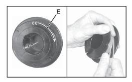
5. Stop when approximately 15-20 cm (6-8 in.) line (C) remains and place ends of line in notches (F) in spool (B).
