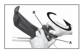
9. Pull both lines out and trim to cut-off knife length.
