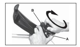
2. Hold drum (A) and turn spool (B) CW (clockwise) until it stops. Pull spool from drum. DO NOT push in on spool when turning.
