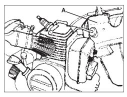
3. Use the brush to remove dirt form cylinder fins.
