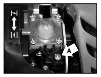
"Specifications" page of this manual. Turn idle screw (A) clockwise to increase idle speed; counter clockwise to decrease idle speed.
