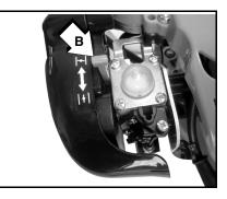
Note: If engine does not start with choke in "RUN" position after 5 pulls, repeat instructions 2 - 5.
