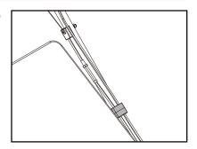
Slip starter handle into loop on 4. handle bar.
