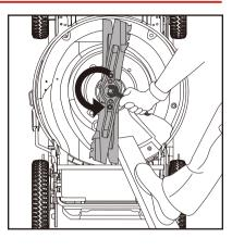
NOTE: Loosen the bolt in counterclockwise direction
