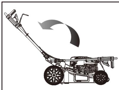
2. Hold down the side bars on both sides of the handle, align with the holes on the sides of machine and release the side bars so that the cylinder latches on the side bars are fixed through the two holes.
