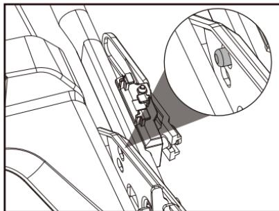
3. Attach the cable to the cable clamp and then attach the cable clamp to the position shown.
