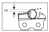
4. File until cutter top and side bevel edges are sharp without nicks.
