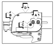
Gently brush debris from inside guide bar cover and from around sprocket.
