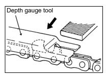
6. Finish cutter sharpening by rounding front raker edge with flat file.
