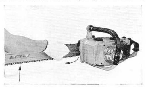
\* Lift the bar end, and tighten the two nuts firmly with a wrench.
