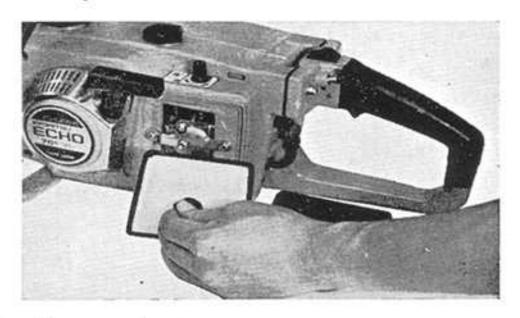
\* Check for any loose screws and nuts of the handles, fan cover and carburetor.
