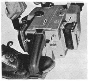
\* Pull the rope 5 or 6 times, and the engine will emit the first firing sound. Next, push the choke button back to the original position. Then pull the rope, and the engine will start.
