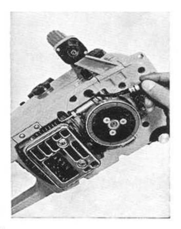
\* If carbon deposits in the cylinder exhaust port and the muffler, the engine output drops and the muffler emitts sparkles.
