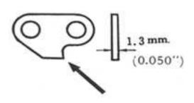
\* The drive links help remove sawdust from the bar grooves. Therefore, sharpen the lower end corner of each link.
