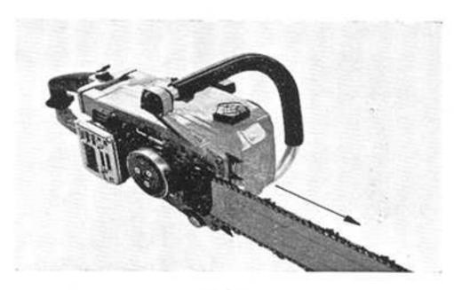
Tension the chain: hold up the bar end by the hand, and turn the adjusting screw clockwise.
