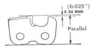
The depth gages limit the cutter depth at the time of cutting.
