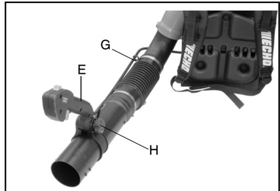
8. Assemble straight pipe w/silencer (I) onto swivel pipe (C), until you feel light resistance. Do not force connection. Hold swivel pipe and turn straight pipe clockwise, engaging positive locking channels, until connection is firm. Do not force connection.
