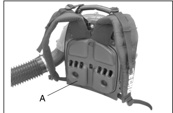
3. Install back cushion (A) to frame over intake cover.
