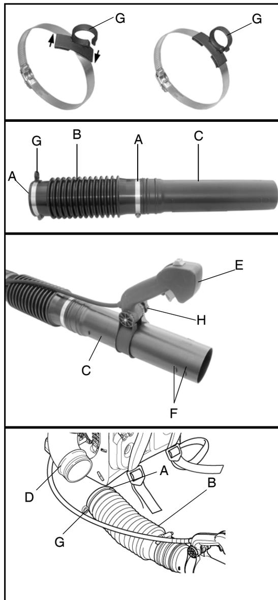
Note: A light lubricant may be used to ease assembly of flexible pipe to blower elbow.
