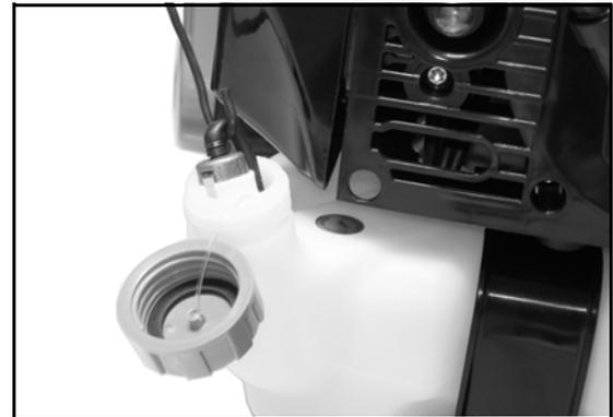
Note: Federal EPA regulations require all model year 2012 and later gasoline powered engines produced for sale in the United States to be equipped with a special low permeation fuel supply hose between the carburetor and fuel tank. When servicing model year 2012 and later equipment, only fuel supply hoses certified by EPA can be used to replace the original equipment supply hose. Fines up to \$37,500 may be enforced for using an un-certified replacement part.
