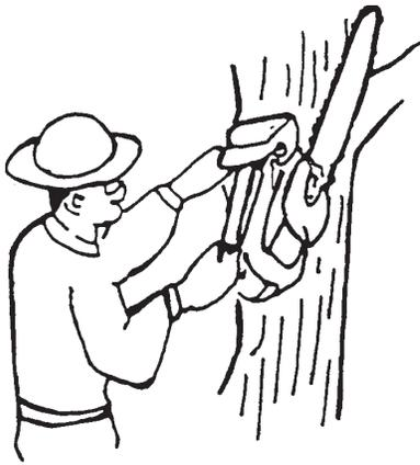
Don't cut with the saw overhead or the bar in a vertical position. If the saw should kick back you may not have good enough control to prevent possible injury.
