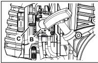
4. Lay the unit on a flat surface and keep movable attachment parts clear of all obstacles. Firmly grasp throttle handle and throttle trigger lockout with left hand and fully depress throttle trigger to wide open position. Rapidly pull recoil starter handle/rope (D) until engine starts (or maximum five pulls).
