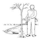
To free a blade that is bound in the cut, stop the engine, and support the trimmer or brushcutter to
