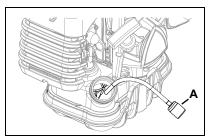
Note: Federal EPA regulations require all model year 2012 and later gasoline powered engines produced for sale in the United States to be equipped with a special low permeation fuel supply hose between the carburetor and fuel tank. When servicing model year 2012 and later equipment, only fuel supply hoses certified by EPA can be used to replace the original equipment supply hose. Fines up to \$37,500 may be enforced for using a replacement part that is not certified.
